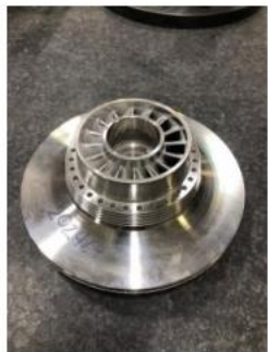
Sage's sCO 2 3MW Turbine Ready for Load Test
