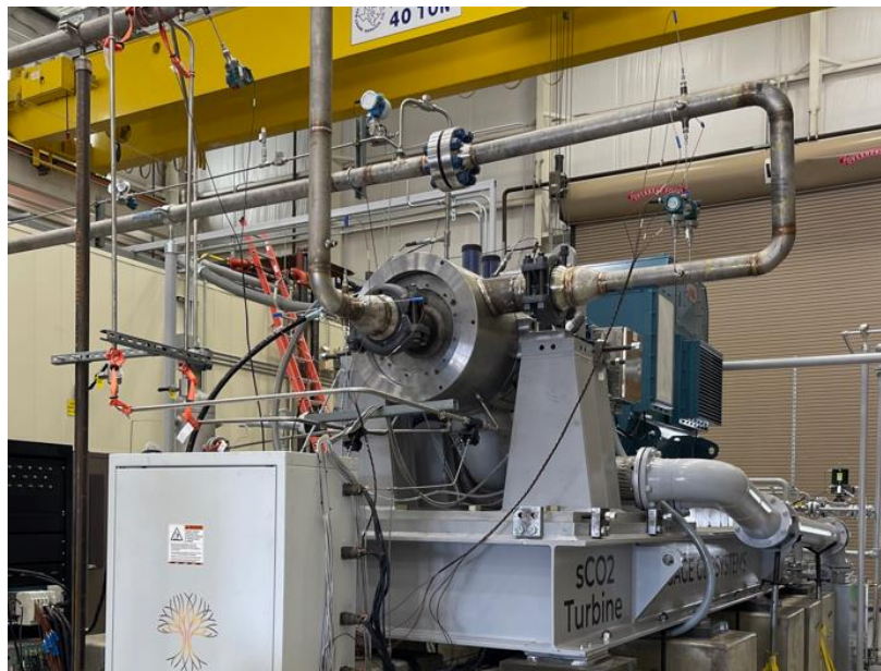
Sage's sCO 2 3MW Turbine Ready for Load Test
