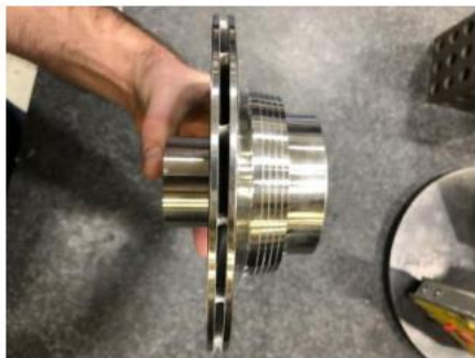
Sage's sCO 2 3MW Turbine Ready for Load Test
